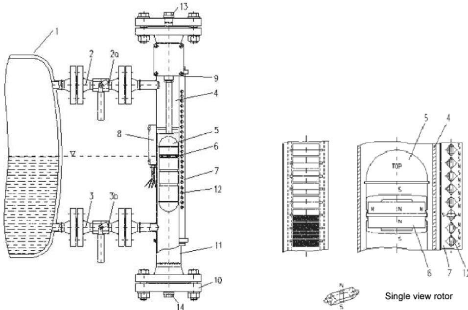
Figure 1: Sectional drawing BNA
