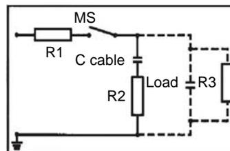
Fig. 1: Protection in case of capacitive loads
