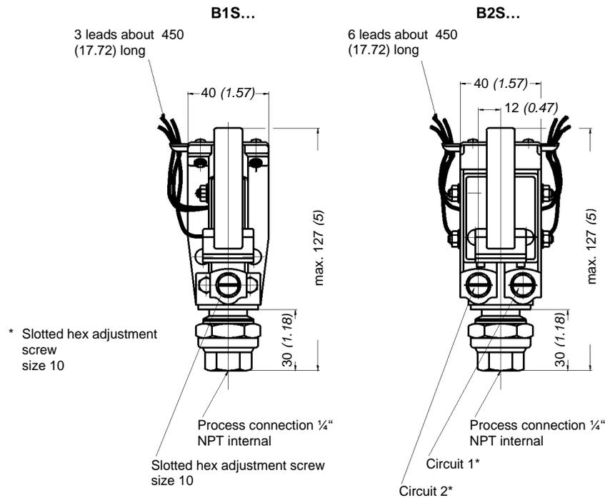
Fig. 7: Bourdon tube pressure switch type B1S .../B2S ...
