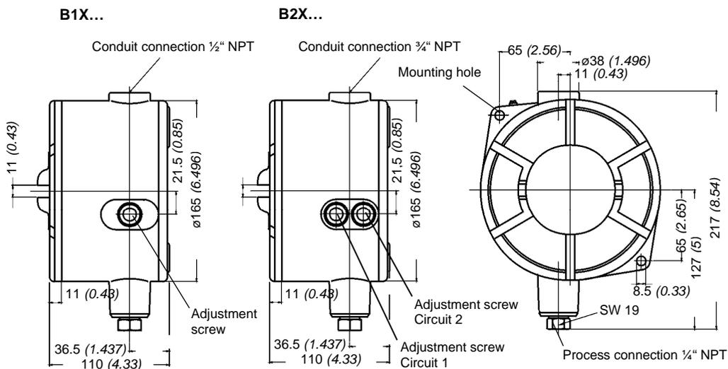
Fig. 10: Bourdon tube pressure switch type B1X .../B2X ...
