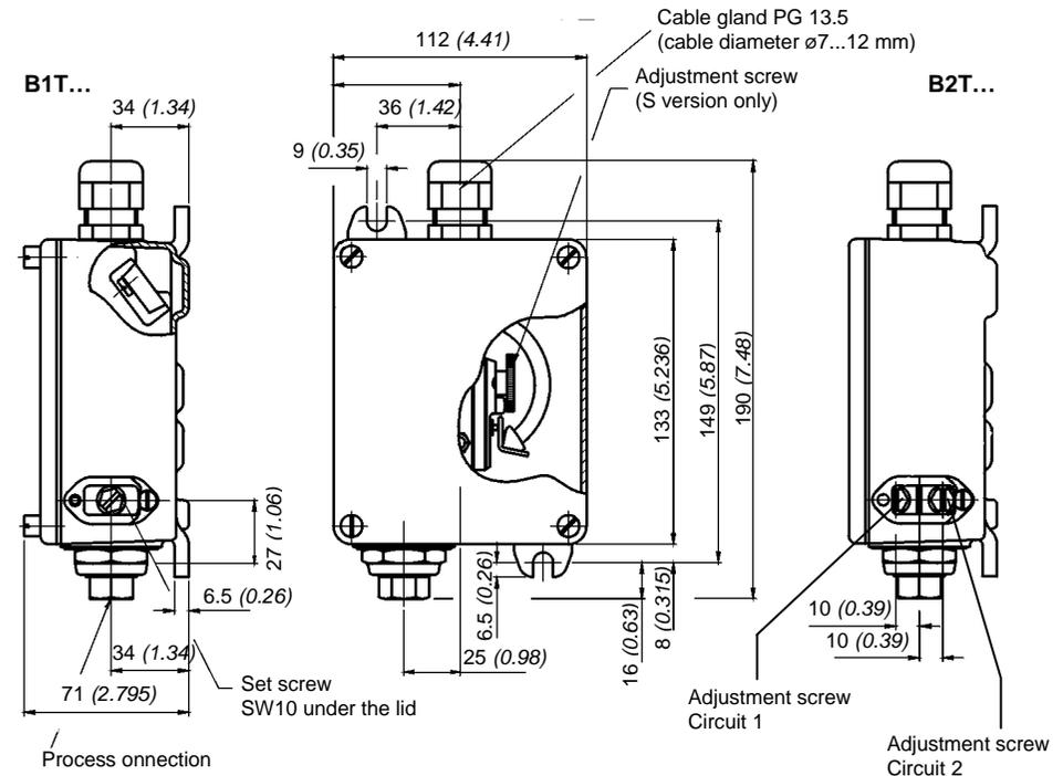
Fig. 8: Bourdon tube pressure switch type B1T .../B2T ...
