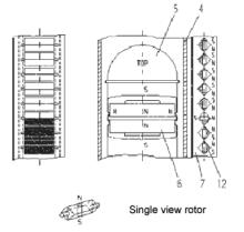
Figure 2: Detail BNA level indicator
