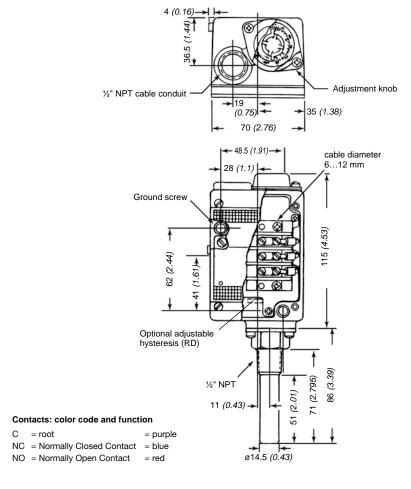
Fig. 11: Temperature switch type ML1H-...
